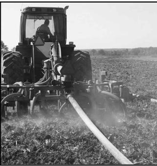
Figure 1 Alkali treated biosolids at 17% solids pumped through a drag hose system
